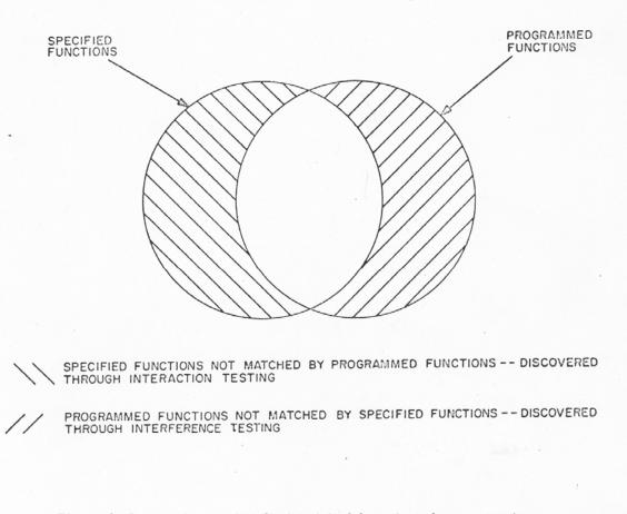
Figure 1. Interaction testing distinguished from interference testing.
